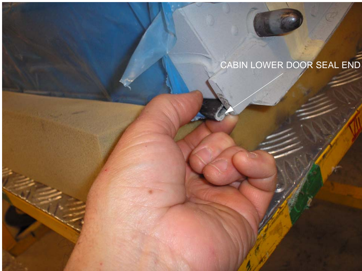
Fig. 205 - Cabin Lower Door Seal Plug - Removal / Installation
