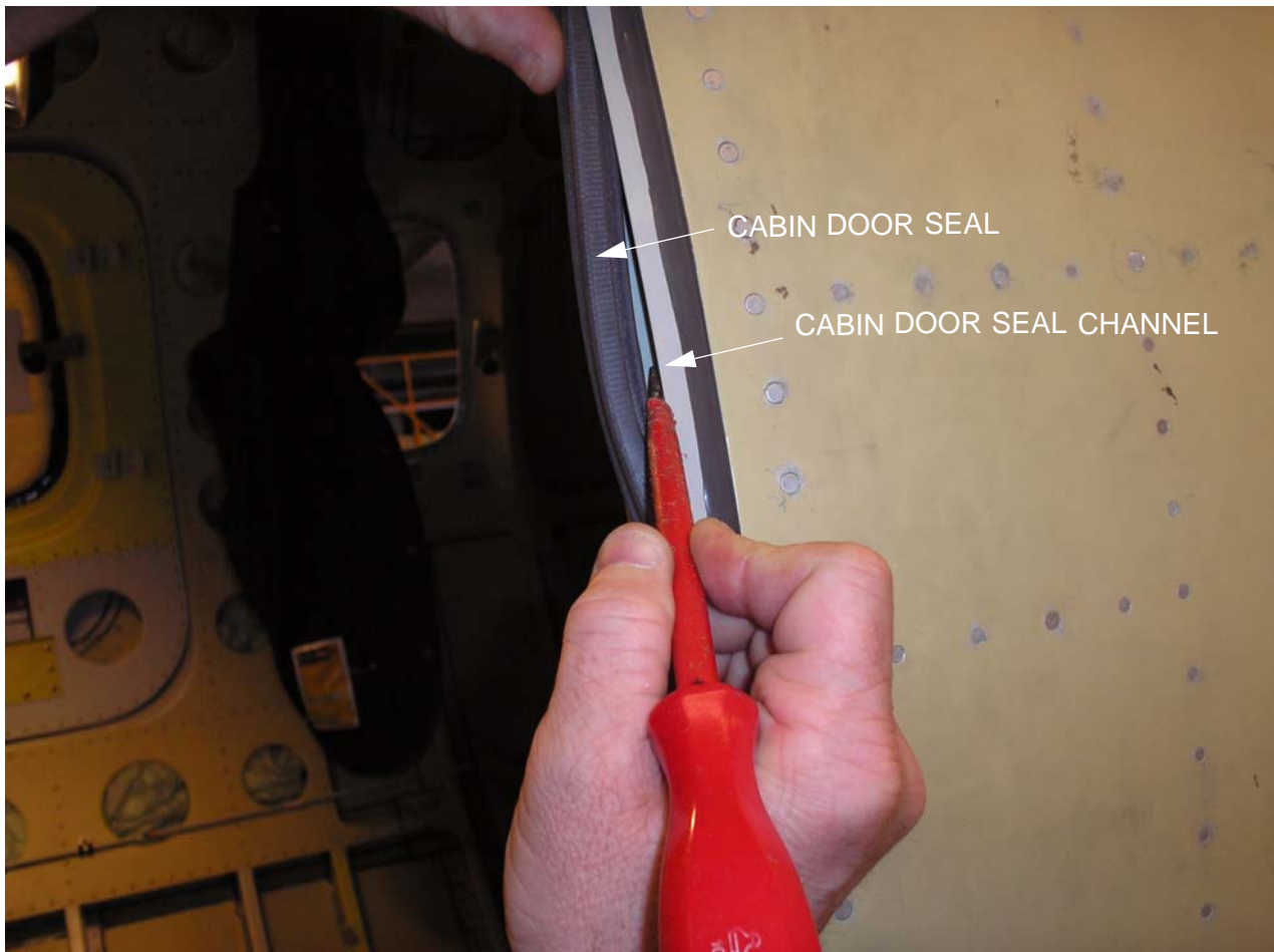
Fig. 201 - Upper Cabin Door Seal - Removal (Sheet 2 of 4)
