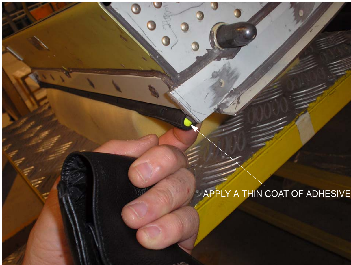
Fig. 205 - Cabil Lower Door Seal Plug - Removal / Installation
