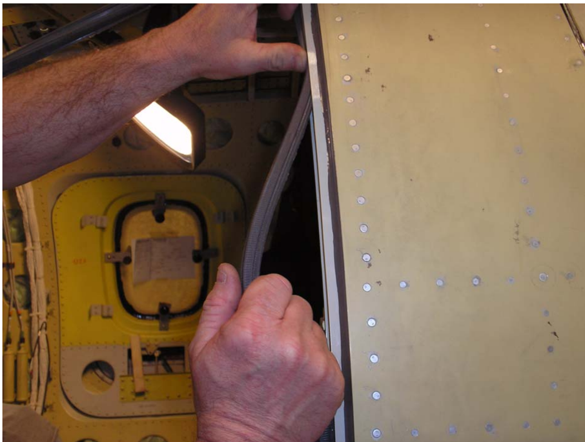
Fig. 202 - Upper Cabin Door Seal - Installation (Sheet 5 of 6)
