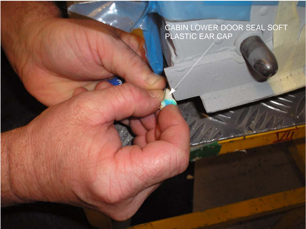
Fig. 205 - Cabil Lower Door Seal Plug - Removal / Installation
