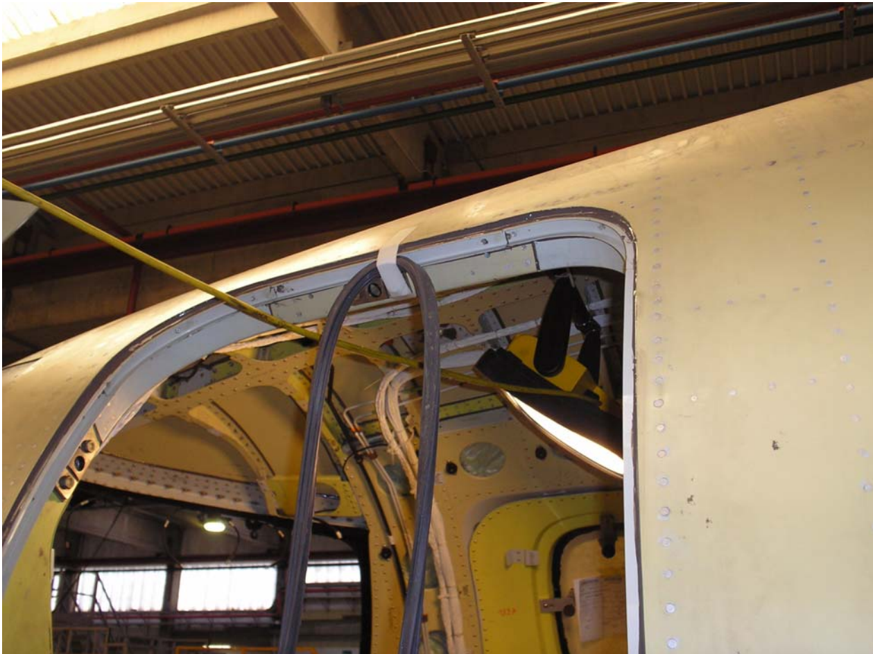
Fig. 202 - Upper Cabin Door Seal - Installation (Sheet 1 of 6)
